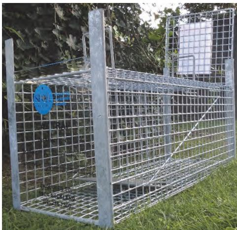
A humane trap is a galvanized steel cage (approximately 8kg in weight) designed to contain an animal without injury. There is a metal sliding door at the entrance with a magnet at the bottom and raised metal bars on each corner to allow the trap door to slide up and down correctly.
